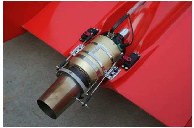
Install vector thrust servos
