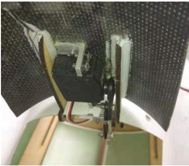
Install air braker servo, open angle 45-70 degree when you open air braker, you need mix elevator up 4mm
